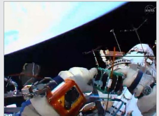
FIGURE 6: Russian cosmonaut preparing to launch a 1U CubeSat that he is holding in his hand. [NASA]
