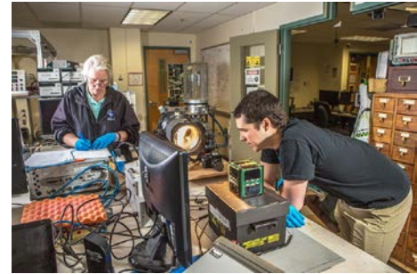
Denise Thorsen and Jesse Frey from the University of Alaska Fairbanks are performing DITL testing on the Alaska Research Center (ARC) CubeSat. ARC was launched by NASA's CubeSat Launch Initiative on the ELaNax XII mission as an auxiliary payload aboard the NROL-55 Mission on October 8, 2015. [University of Alaska, Fairbanks]
