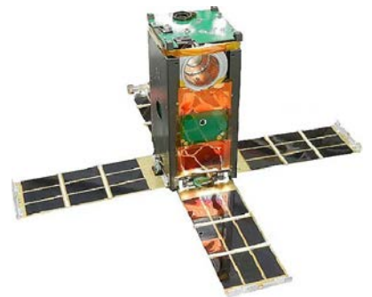
CXBN, the Cosmic X-Ray Background NanoSat was developed and built by students from Morehead State University in Kentucky. Its primary purpose is to increase the precision of measurements of the Cosmic X-Ray Background in the 30–50 KeV range. Launched by NASA's CubeSat Launch Initiative on the ELaNa VI mission as an auxiliary payload aboard the NROL-36 Mission on November 13, 2012. [Morehead State University]
