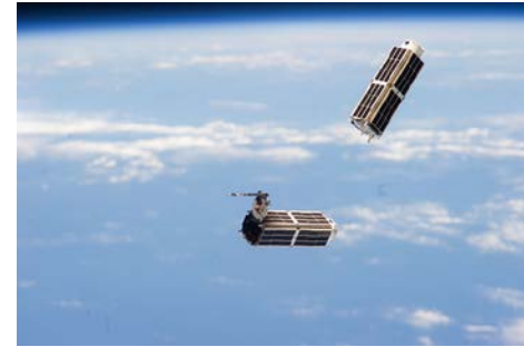
A set of NanoRacks CubeSats is photographed by an Expedition 38 crew member after the deployment by the Small Satellite Orbital Deployer (SSOD). [NASA]
