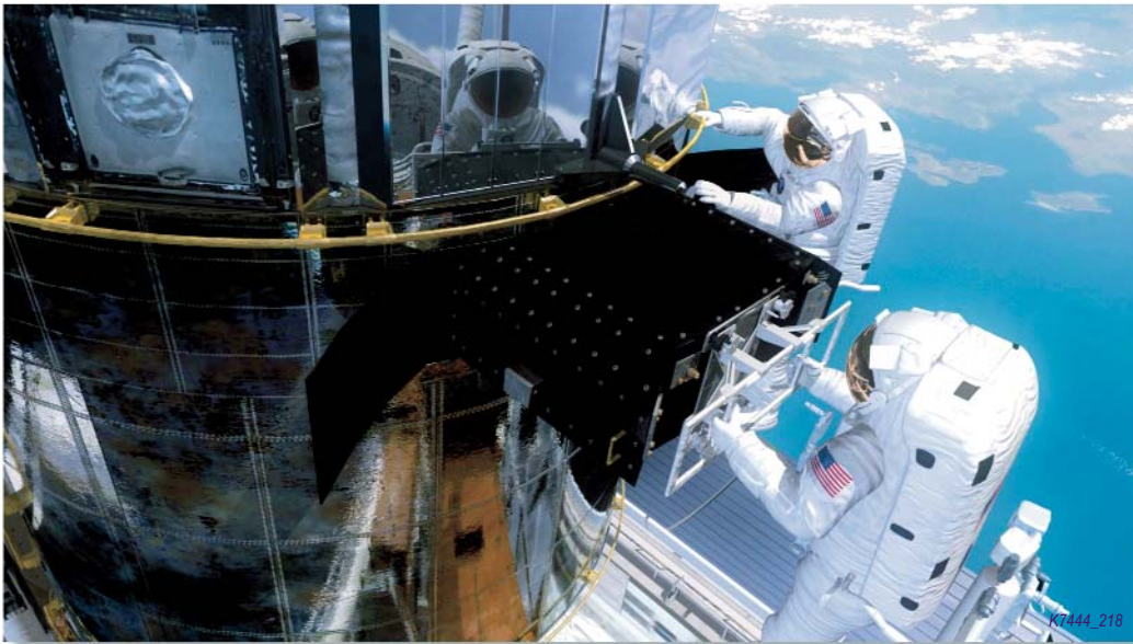
Fig. 2-17 Andrew Feustel moves a refurbished Fine Guidance Sensor into position on Hubble with assistance from John Grunsfeld, to his right.
