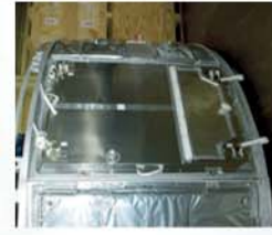
New Outer Blanket Layer (NOBL) insulation Onto Bays 5 and 8
