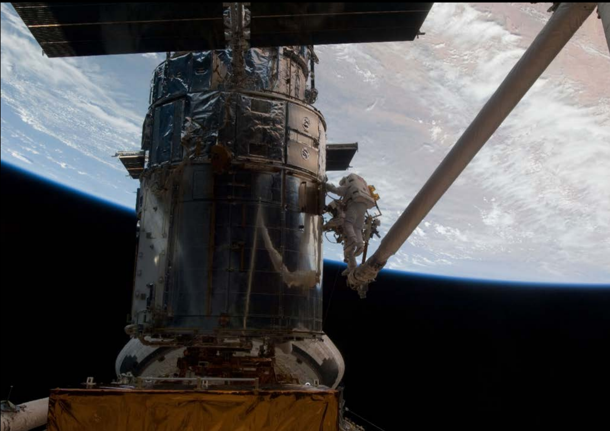
Astronauts John Grunsfeld and Andrew Feustel replace a Fine Guidance Sensor on Hubble during the last servicing mission in May 2009.
