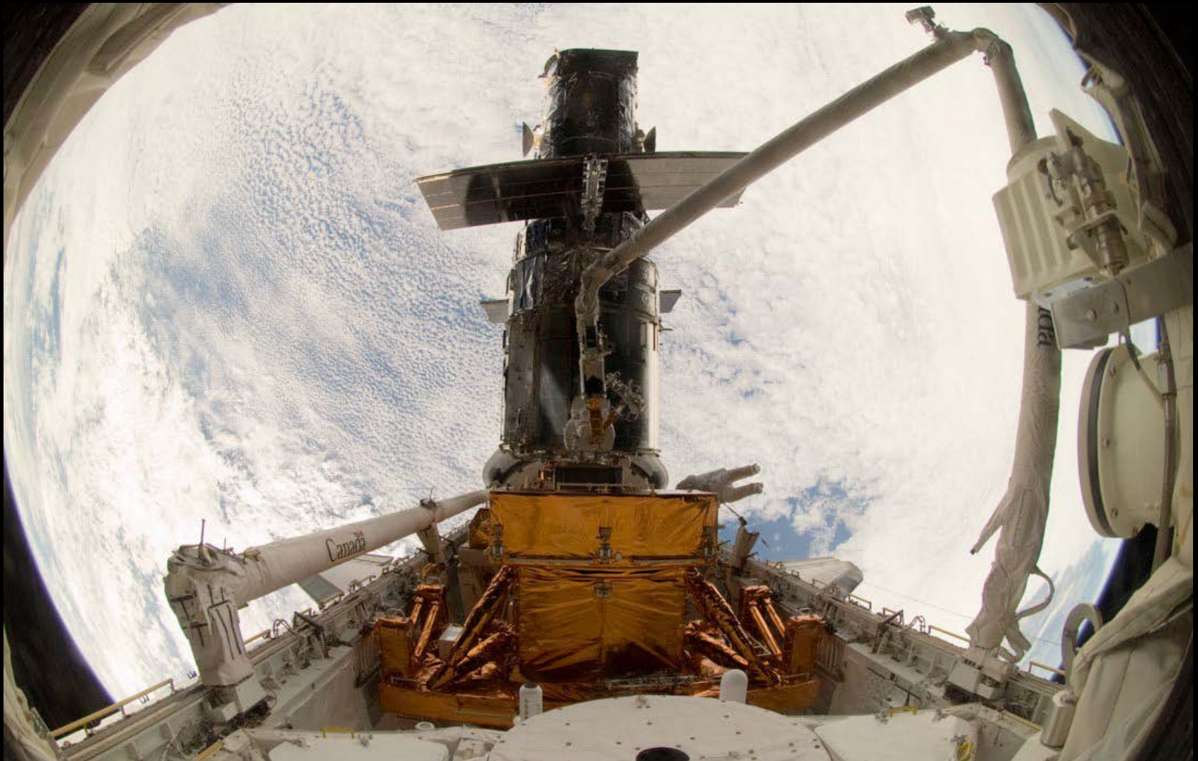
Astronauts John Grunsfeld and Andrew Feustel install a new Fine Guidance Sensor on Hubble during the last servicing mission in May 2009.
