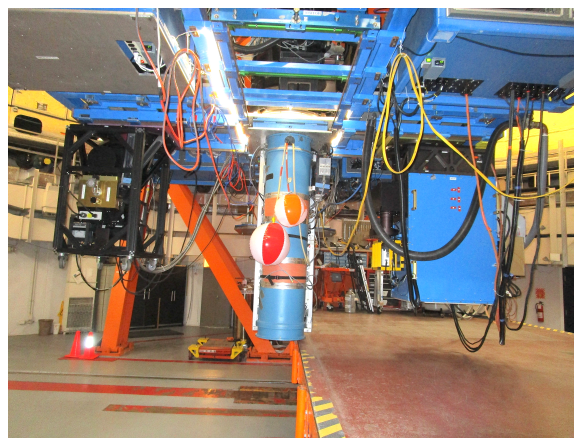
Figure 5. TEXES in the on-axis observing location. MIRSI (left) and SpeX (right) are in their west and east stow positions respectively.
