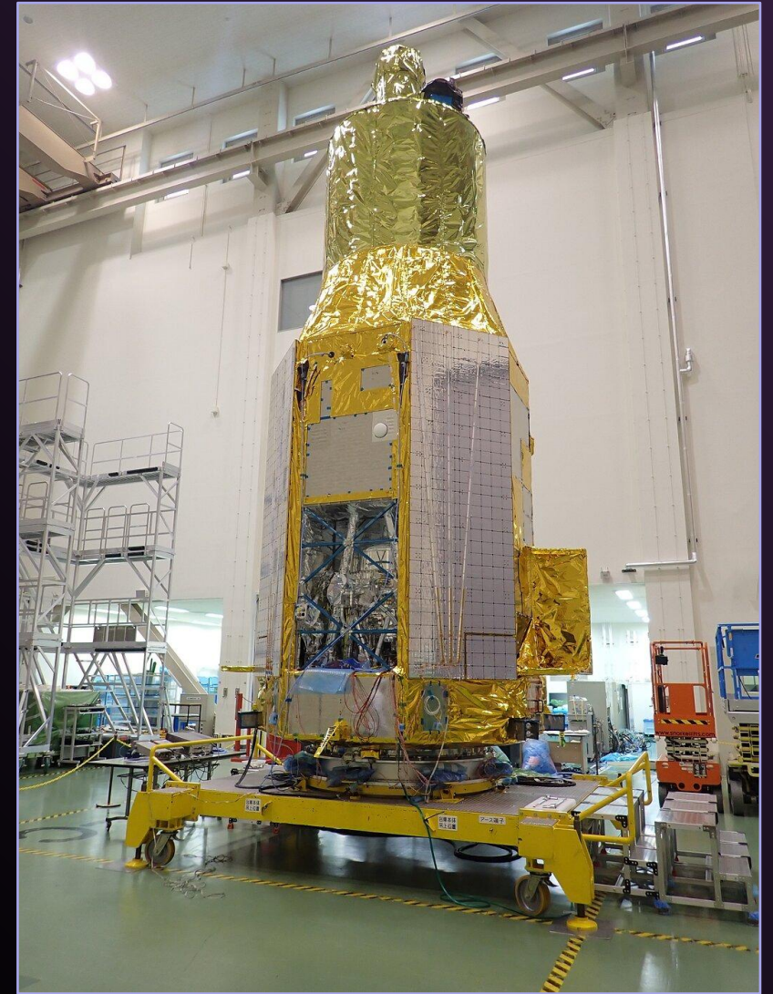
The XRISM spacecraft as it appeared in May at Tsukuba Space Center, Japan. The open compartment near the bottom houses its Goddard-developed Resolve instrument. Credit: JAXA/NEC
