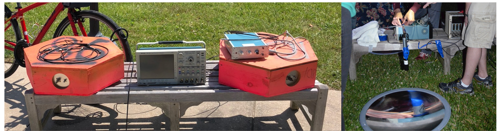
Muon and Cherenkov detectors reveal cosmic-ray showers
