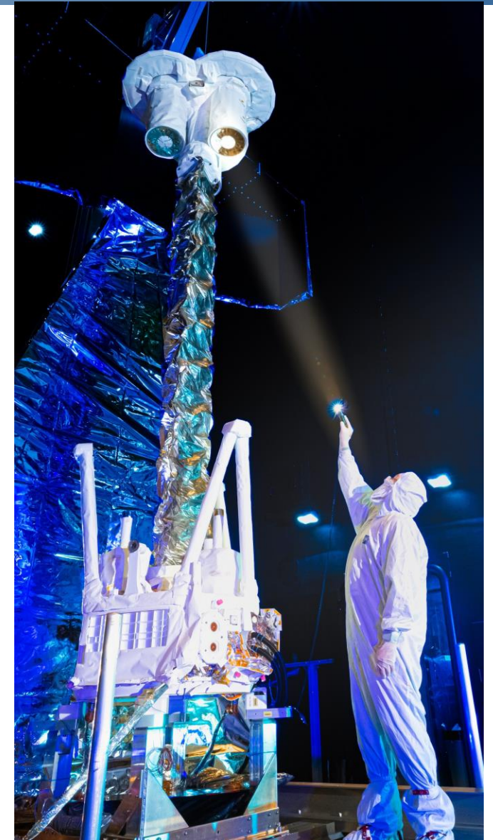
IXPE during environmental testing at Ball Aerospace
