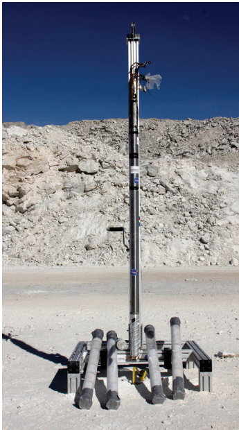
An initial version of the drill technology—the Auto-Gopher-1—is pictured here with cores it acquired from drilling a 3-m hole in 40 MPa gypsum.
