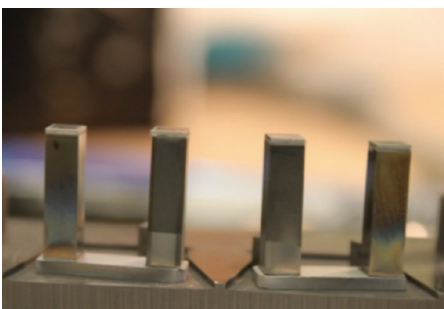
Left: New industry-produced SKD couples that are resilient enough to operate in the eMMRTG hermetically sealed convertor cavity. (Credit: S. Keyser, Teledyne Energy Systems, Inc.) Center: Monte Carlo simulation of heat flow across composite TE material with metal inclusions. (Credit: P. von Allmen, JPL/Caltech) Right: High-temperature segmented thermoelectric module technology with 2X efficiency gain over heritage RPS technology. (Credit: S. Firdosy, JPL/Caltech)
