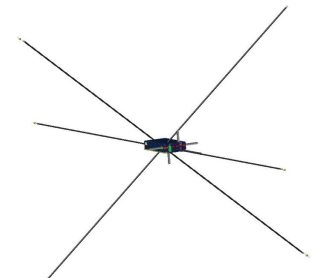
Left: Electric field booms compactly stowed in the CubeSat volume (10 cm on a side). Right: Six booms extend sensors from the main CubeSat body to distances of 5m, tip-to-tip, enabling tri-axial or vector electric field measurements. (Credits: CTD and NASA GSFC)
