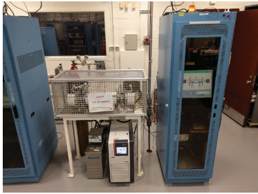
TDCs #13 and #14 on extended operation in the Stirling Research Lab. (Credit: NASA Glenn Research Center)
