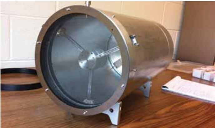
The laboratory prototype of the NDA instrument
