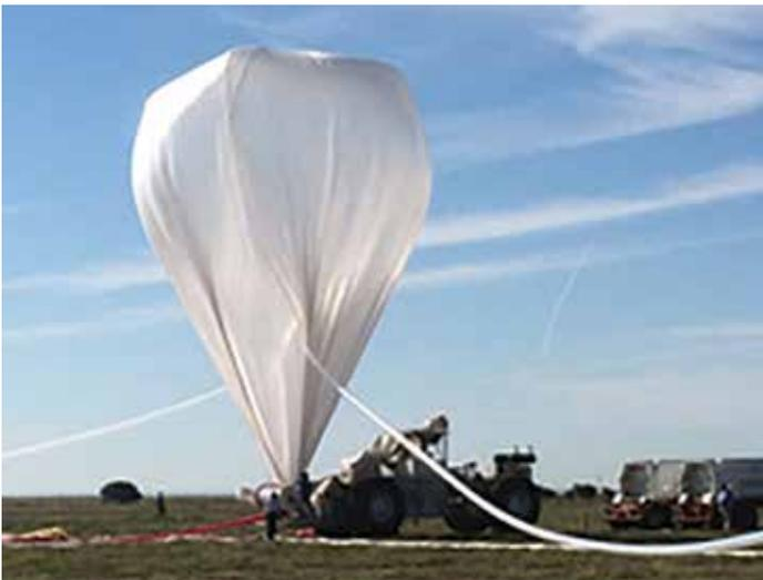
A NASA high-altitude balloon is inflated with helium in preparation for the HySICS science demonstration flight. (Image: NASA Balloon Program Office.)
