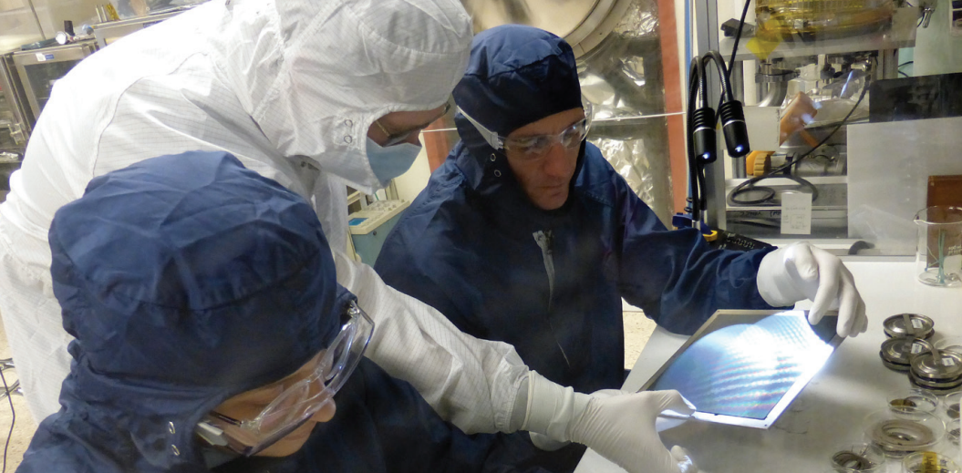
▶ Team members inspecting a 20 cm atomic layer deposited microchannel plate (left). Cross strip imaging readout anode (right).
