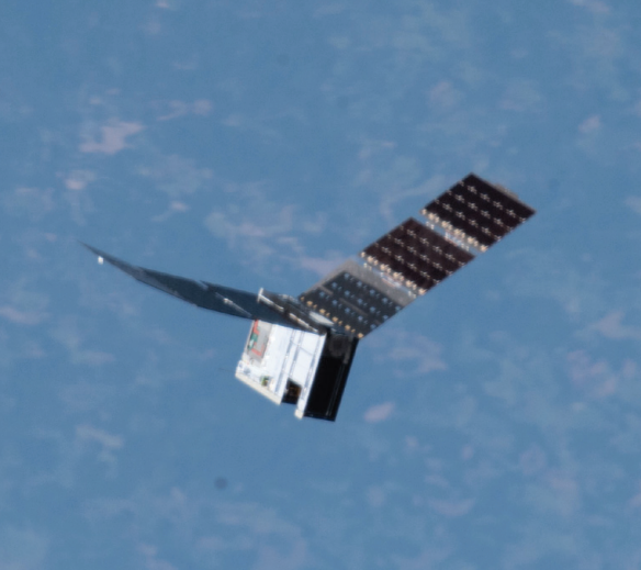
► The TEMPEST-D CubeSat after deployment from the International Space Station (ISS) on July 13, 2018 (left). Shortly after becoming fully operational, TEMPEST-D captured this first full-swath image of Hurricane Florence on September 11, 2018 (right). The colors reveal the eye of the storm, surrounded by towering, intense rain bands. (Visual image of the storm clouds on right taken by the National Oceanic and Atmospheric Administration's [NOAA] Geostationary Operational Environmental Satellite [GOES]; NASA/NOAA/Naval Research Laboratory Monterey/JPL-Caltech)
