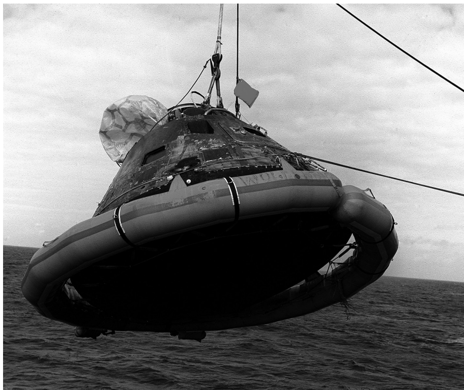
Figure 4.4 Apollo 11 Command Module and its flotation collar hoisted aboard the USS Hornet . Astronauts have already exited from the craft.
