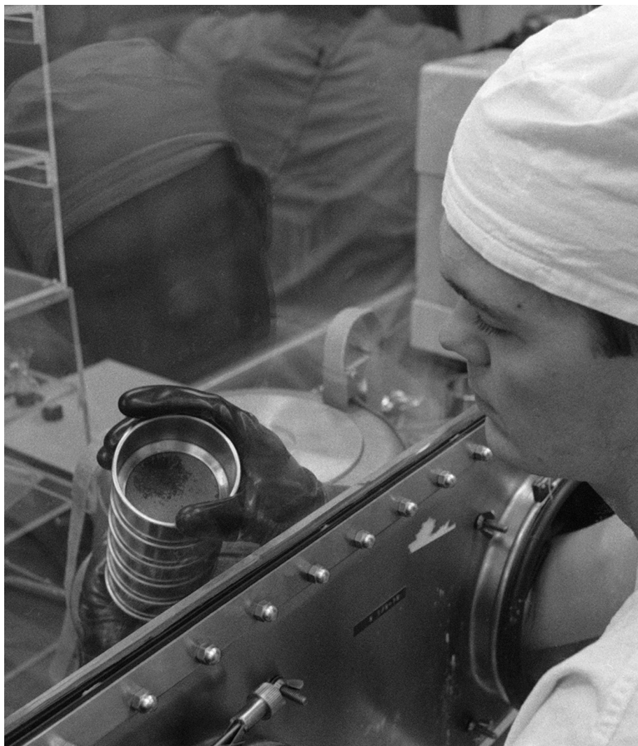
Figure 4.9 Lunar material in a sieve from the bulk sample container being examined in an LRL glove box by a lunar sample preliminary examination team member.
