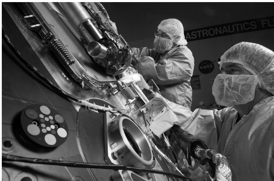
Figure 7.2 Phoenix spacecraft assembly, with Lockheed Martin Space Systems technicians working on the science deck of the Phoenix Mars Lander. Assembly operations took place in a class 100,000 cleanroom with NASA's planetary protection practices being strictly followed to prevent organics from being transported to Mars. The lander's robotic arm, built by JPL, is at the top.
