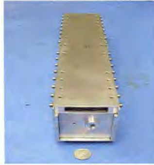
Figure 2.3-6. MER Li-Ion Battery
