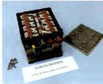
Figure 2.3-1. Mars Pathfinder Silver Zinc Battery
