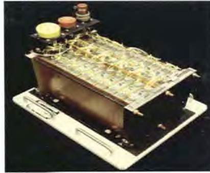
Figure 2.3-2 TOPEX Ni-Cd Battery
