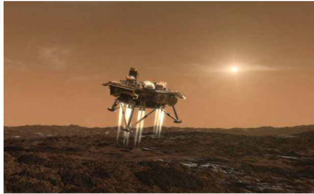
Figure 3.1.1-1. A Phoenix-derived Mars Sample Return (MSR) concept shown performing precision landing on Mars in an artist's concept.
