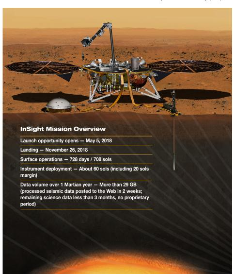
InSight is based on the proven Phoenix Mars spacecraft and lander design with state-ofthe-art avionics from the Mars Reconnaissance Orbiter and Gravity Recovery and Interior Laboratory missions.
