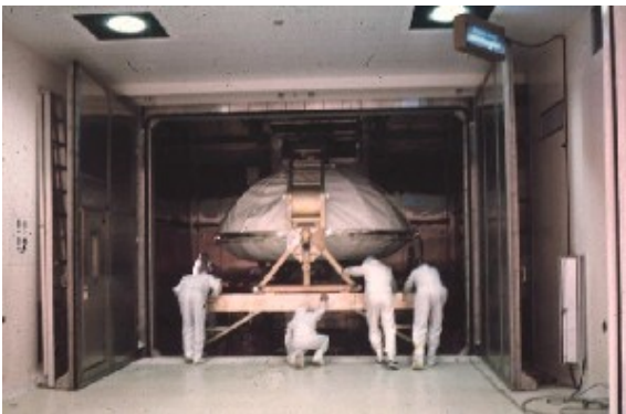
Figure 3-7. Viking engineers preparing the spacecraft for sterilization.
