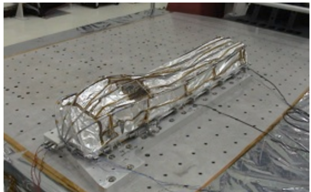
Figure 3-8. The Phoenix bio-barrier. The robotic arm is shown encased in the bio-barrier, held in place by a series of latches released shortly after landing by a pyro-activated pin puller. Torsion springs at each end then rotated the ribs (right to left in the figure) to open the enclosure [77].
