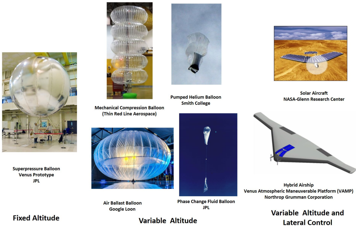
Figure 3-1 Venus Aerial Platform Concepts considered in this study are subdivided into three categories: Fixed Altitude platforms, Variable Altitude platforms as well as Platforms with both Variable Altitude and Lateral Control.
