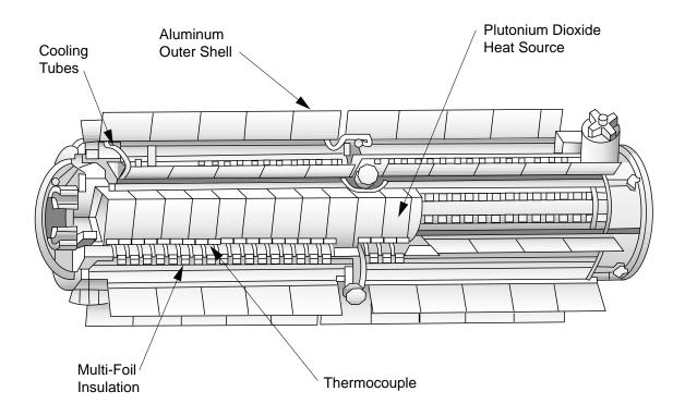
Radioisotope thermoelectric generator (RTG)
