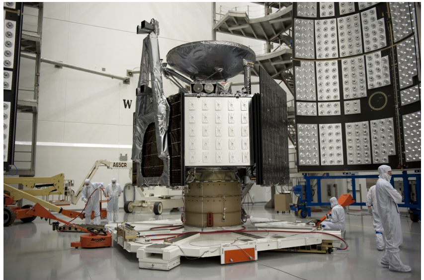
Five of Juno's six MWR antennas are located on one side of the spacecraft. The largest of Juno's six MWR antennas takes up a full side of the spacecraft.
