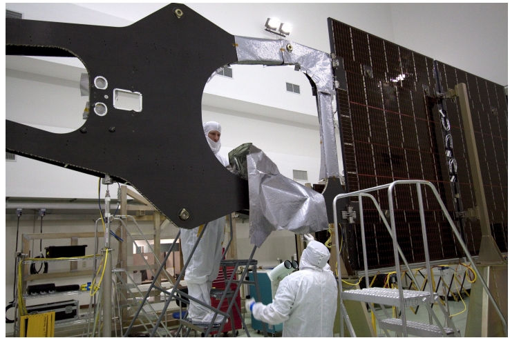
Thermal blankets being installed on Juno's magnetometer boom. Credit: NASA
