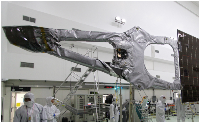
Juno's two magnetometers are located on a boom at the end of one of its long solar arrays.
