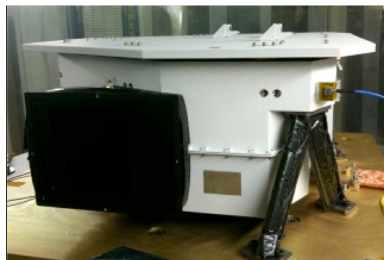
JIRAM is an infrared spectrometer designed to observe Jupiter's auroras and atmosphere from very close to the planet.
