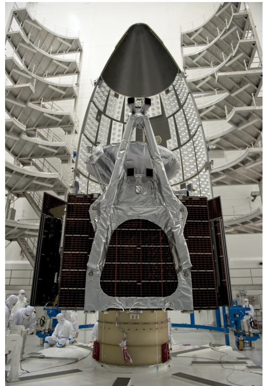
Four star tracker cameras help determine the precise orientation of the magnetometers as they sense Jupiter's magnetic field.
