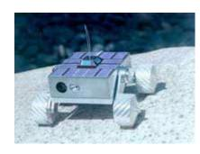
The MUSES-CN nanorover will be the smallest rover ever to fly on a space mission. (MUSES stands for the Mu Space Engineering Spacecraft--which is being built by the Japanese Institute of Space and Astronautical Science--C means it is the third in a series, and N stands for NASA's part in it, which is to build the nanorover.)
