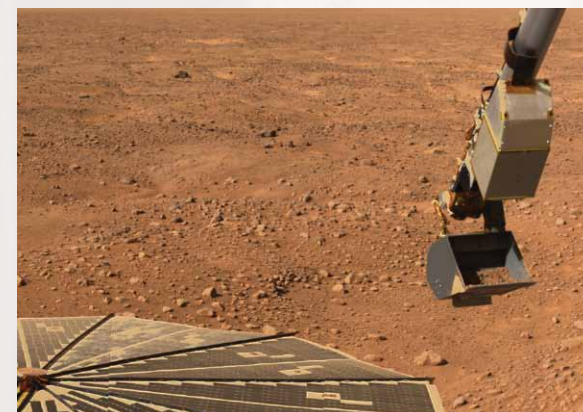
This image shows NASA's Phoenix Mars Lander's solar panel and robotic arm with a sample in the scoop. The image was taken by the lander's Surface Stereo Imager on June 10, 2008. Credit: NASA/Jet Propulsion Laboratory-Caltech, University of Arizona, and Texas A&M University.
