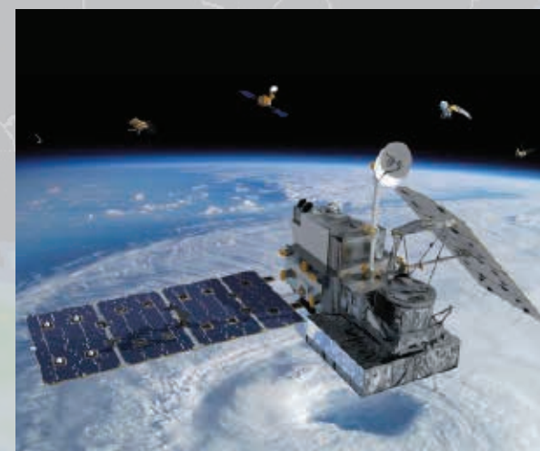
Artist's rendering of the GPM Core Observatory [foreground] with constellation satellites [background]. Image credit: NASA
