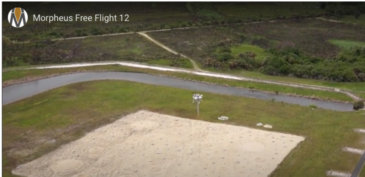
Figure 14. Morpheus demonstration of onboard hazard detection and avoidance showing the terminal portion where the ALHAT onboard Hazard Detection System (HDS) identifies a safe landing site 1.4m east of the pad center and diverts to land at that location. (credit: https://youtu.be/tmkPJUHdRA )
