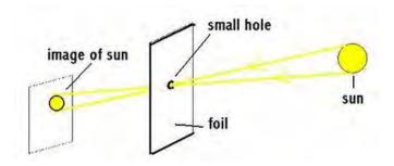
A solar viewer, or pinhole viewer, works by projecting the image of the sun onto a surface behind the small hole. The smaller the hole, the sharper the image will be. Light rays from the top of the sun go to the bottom of the image and light from the bottom of the sun creates the top of the image. The image you see is actually upside-down, but because the Sun is basically symmetrical, this effect is not noticeable.
