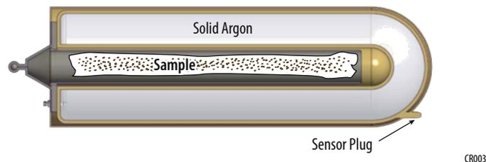
Figure 3-5: Cryogenic Sample Dewar
