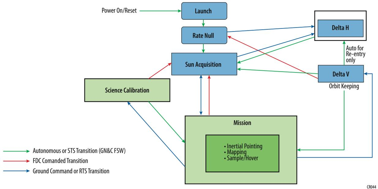
Figure 7-2: GNC Mode Diagram
