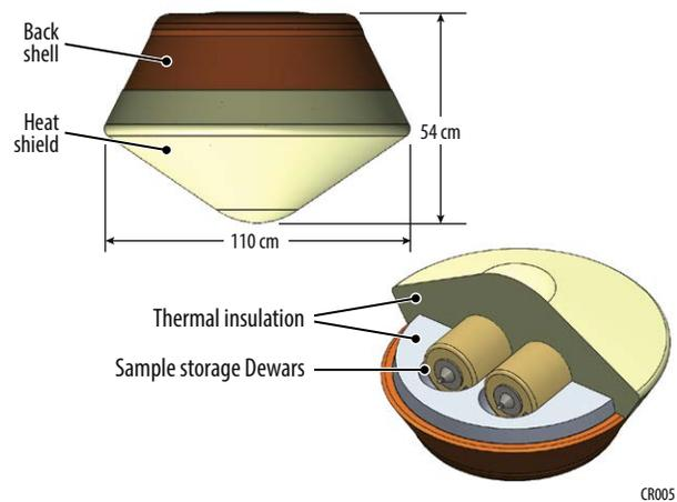
**Figure 3-6: Earth Entry Vehicle with Sample Storage Dewars**
