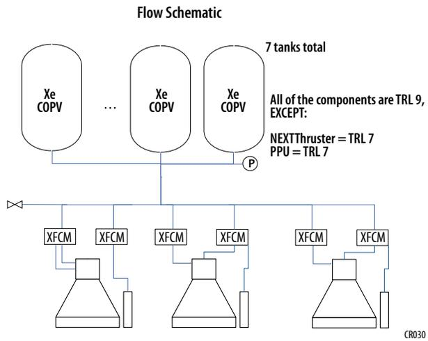
**Figure 6-2: SEP System Flow Schematic**
