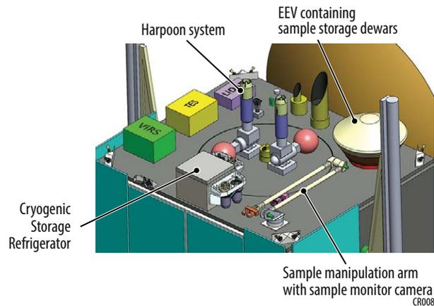
**Figure 3-3: Cryogenic Sample Chain**
