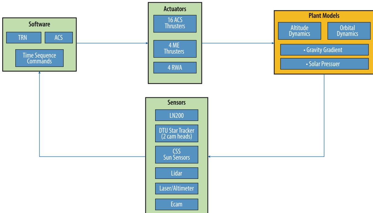
Figure 7-1: GNC Block Diagram
