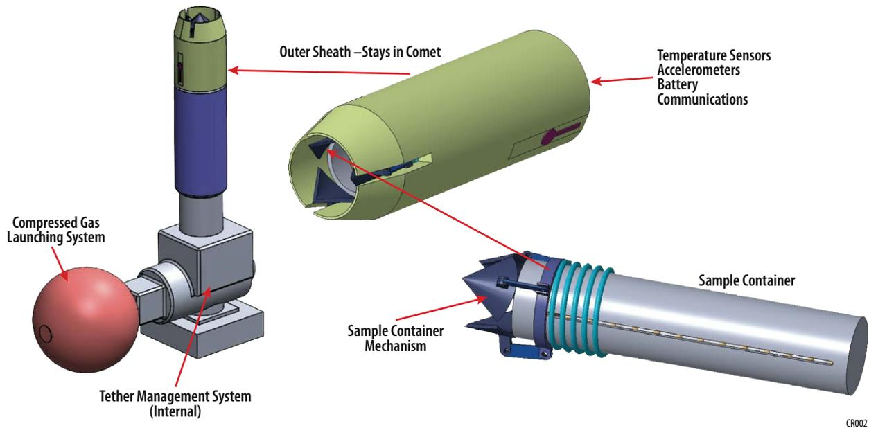
**Figure 3-4: Harpoon Sample Acquisition System**
