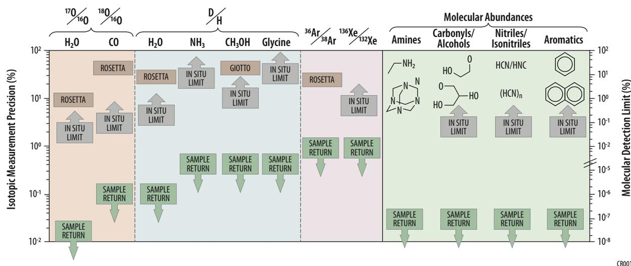
**Figure 1-1: Volatile measurement capabilities for returned samples are superior to those for in situ spacecraft. Here examples for a comet are shown Left: isotopic measurement precision for selected volatiles. Right: molecular detections for selected classes of organics. Reprinted from Milam et al., (2020).**
