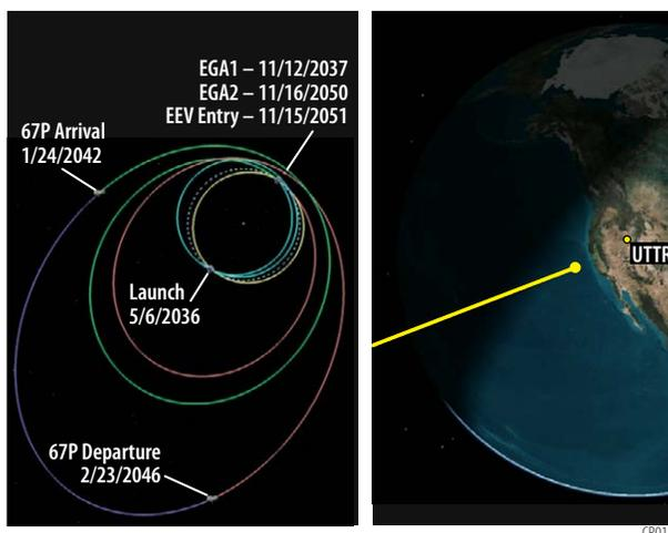
**Figure 3-7: Left: Top-down view (from ecliptic north) of CROCODILE's SEP trajectory. The different legs of the trajectory are shown in various colors to distinguish them on the plot. Earth's orbit is shown for reference as a dashed line. Right: EEV approach up to atmospheric entry interface at a radius of approximately 6532 km. Target landing site at UTTR**
