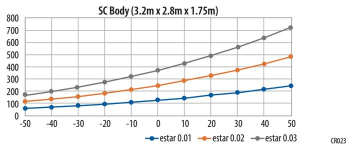
Figure 4-1: Heat Loss Thru MLI
