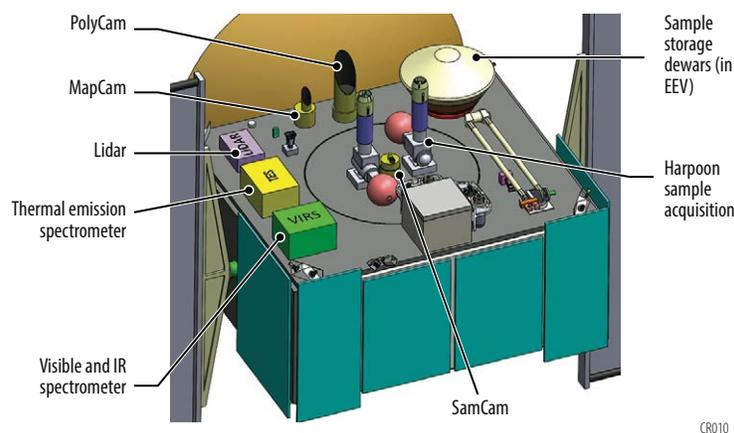
**Figure 3-1: Instrument Payload Layout**
