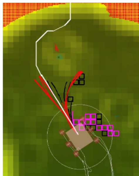
Figure 16. A view of the ENav simulation environment. The green-yellow terrain shows how the Gradient Convolution heuristic, developed in this work, has assessed the cost of traversing the terrain (yellow regions are higher cost) and steers the rover toward safer regions.
