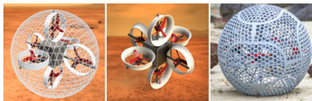
Figure 6. Left: Rollocopter concept art, including propellers, electronics (gray box), and the impact-resilient cage. Middle: Hexacopter configuration of the propellers. Right: A Rollocopter prototype.
