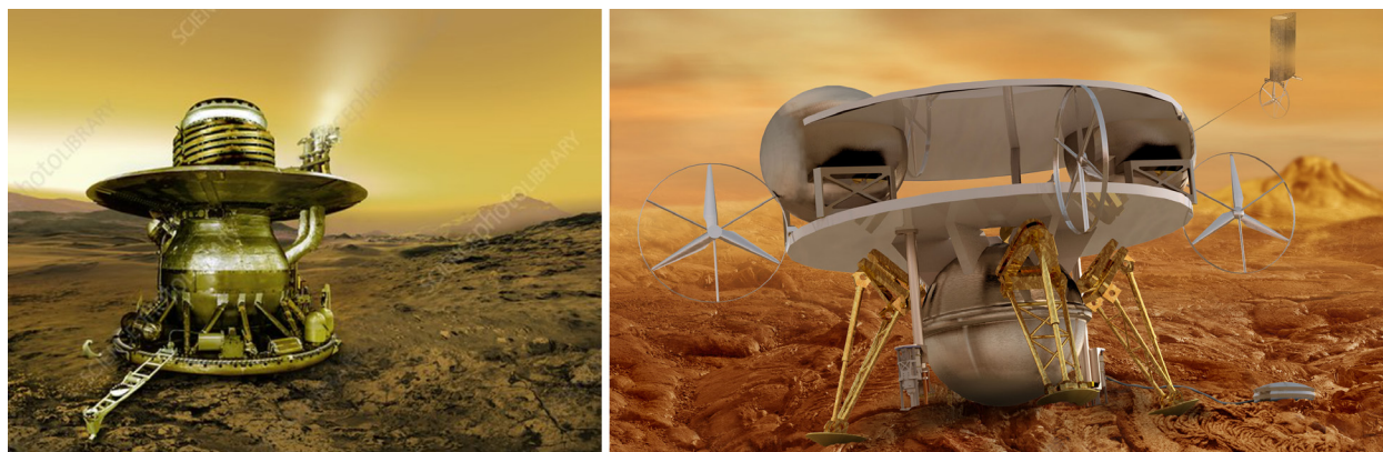
Figure 5. Venus landers must employ aerodynamic control during final descent because rocket propulsion is not effective at the high atmospheric density of the Venus surface. The Soviet-era Venera landers (left, courtesy Detlev van Ravenswaay/Science Photo Library) used a circular drag brake to arrest the speed of descent and assure safe landing. For landing in more hazardous terrains where surface wind velocities are higher, rotorcraft approaches (right) are being considered. 31
