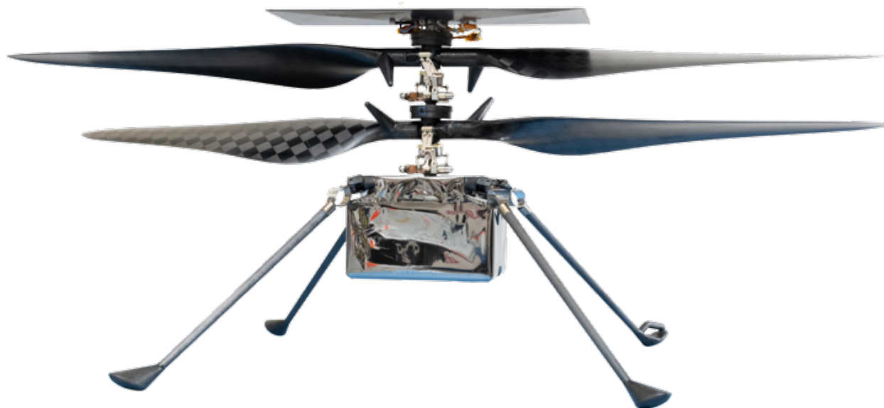
Figure 13. The Mars Helicopter, Ingenuity, has two coaxial counter-rotating rotor blades and is powered by batteries that are recharged with solar power when the helicopter is on the surface of Mars. (Courtesy NASA/JPL-Caltech.)
