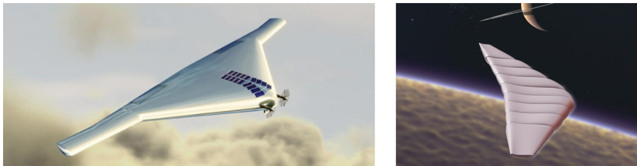
Figure 22. The VAMP vehicle (left) is powered by solar panels in the upper side of the wings and exploits both buoyancy and aerodynamic lift (credit: Northrop Grumman). The T-LEAF vehicle (right) has no propulsion system but uses changes in buoyancy to maneuver (credit: Global Aerospace Corporation/Northrop Grumman Aerospace Systems).
