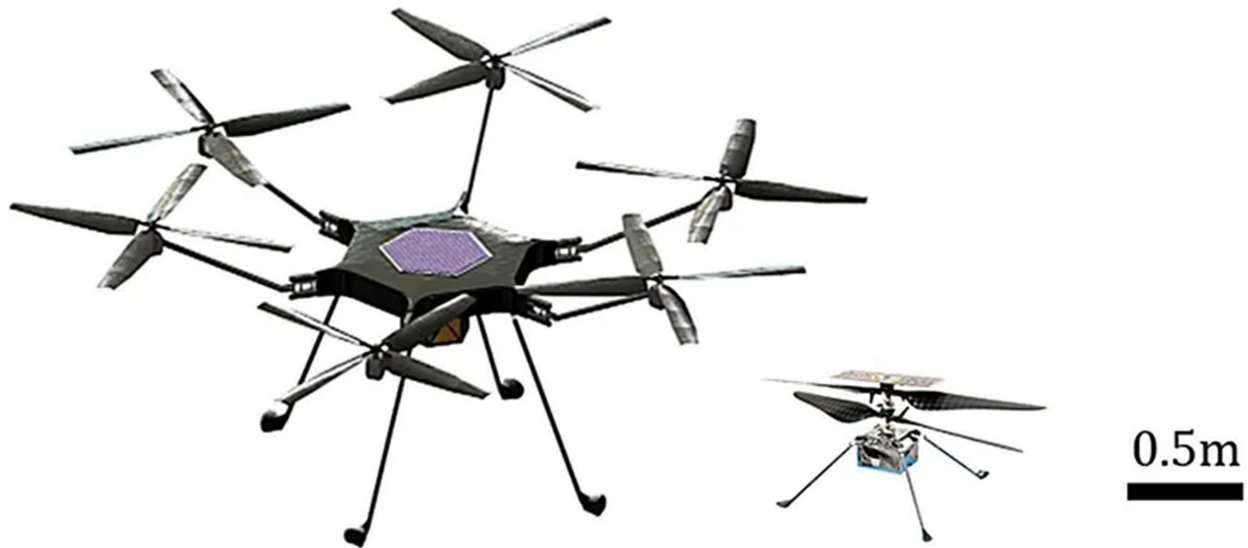
Figure 15. The MSH takes advantage of the validation of the performance of the rotors on Ingenuity. Each MSH rotor is the size of an Ingenuity rotor. 17
