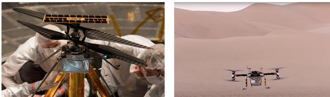
Figure 24. Left: Testing of the Mars Helicopter, Ingenuity, required a large vacuum chamber to represent the low-pressure environment at Mars (courtesy NASA/JPL-Caltech). Right: These tests of Dragonfly take advantage of outside flight in a dune environment morphologically representative of that found on Titan (courtesy NASA/Johns Hopkins APL).
