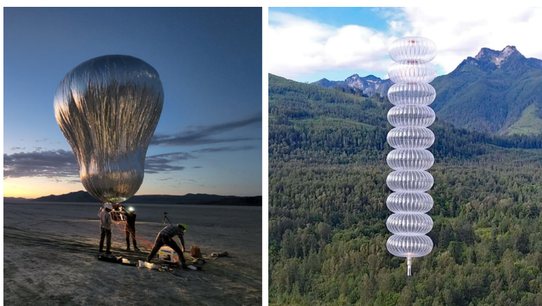
Figure 4. Two approaches to a variable-altitude aerobot, both using helium compression to modulate the volume of the buoyant chamber. The pumped compression balloon (left) pumps helium between a pressurized inner balloon and a zero-pressure outer balloon (courtesy NASA/JPL-Caltech). The mechanical compression balloon (right) uses a tether to compress the entire balloon volume (courtesy Thin Red Line Aerospace).
