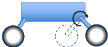
Figure D-2. Four-wheeled skid vehicle with active suspension (amenable to walking)
