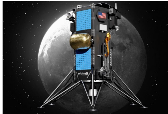
Figure H-2. PRIME1 mission. TRIDENT is vertically mounted on the right hand side of the Intuitive Machines (IM) lander.
