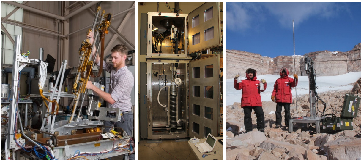
Figure D-16. Left: TRIDENT drill undergoing TVAC tests at NASA GRC. Center: Icebreaker drill in Mars chamber. Right: Icebreaker drill undergoing testing in Antarctic Dry Valleys.
