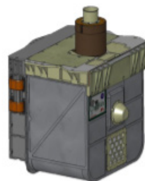
Figure 1: The MSL CheMin instrument (left) and 2D XRD data (right). Resolution is \sim 0.3^\circ 2\theta .
