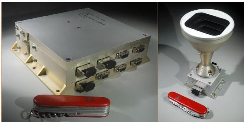
Figure 9: MSSS ECAM 50 DVR (left) and camera head (right).
