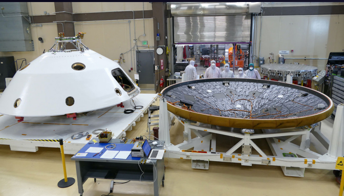
Below: MEDLI2 sensors installed on Mars2020 heat shield and back shell
