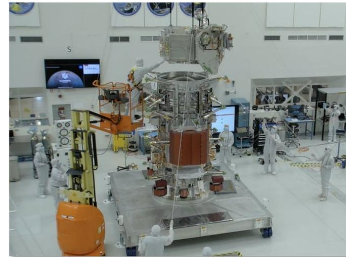
*Avionics module atop the propulsion module*
