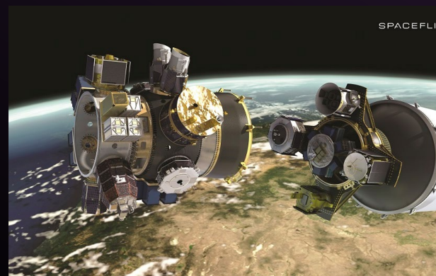
SPA-Ring Payload Port Limit (450 kg)
