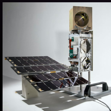
CubeSat/Nanosatellite TROPICS 3U/6U (1 – 10 kg)
