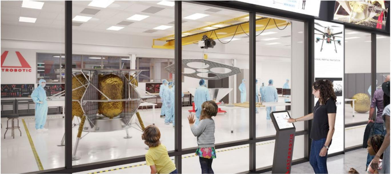
Astrobotic's Lunar Logistics Headquarters contains two ISO Class 8 cleanrooms capable of hosting four concurrent spacecraft for payload and lander integration and has an adjoining mission control center.
