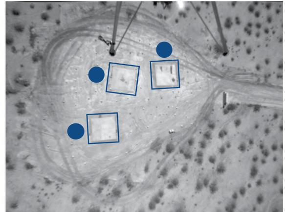
Early version of the OPAL sensor autonomously selects a hazard-free landing site for the Masten Space Systems Xombie Rocket.
