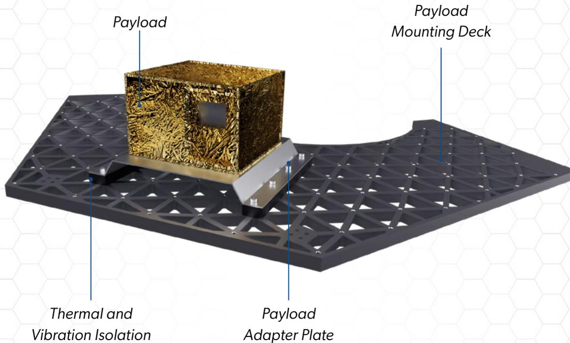
Additionally, the adapter plate can be utilized to dampen loads as experienced by the payload. It can also simplify the provision of the required thermal characteristics as well as the implementation of the required grounding, bonding, and isolation techniques at the payload mounting interface to the lander.
