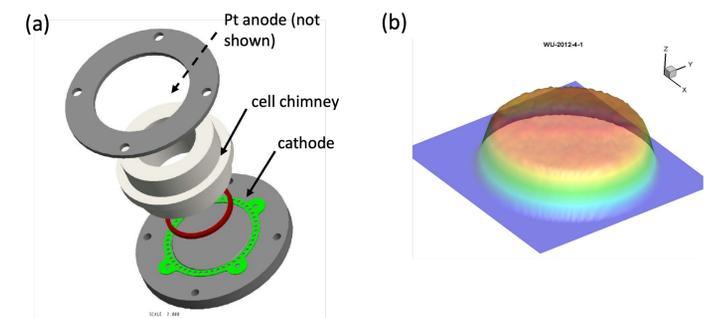
Fig. 5: (a). Exploded view of electroplating cell. The plating substrate is attached to the green ring. <sup>244</sup>Cm is electroplated onto the substrate from a dilute solution of Cm in isopropanol. (b). Source Intensity <sup>3/4</sup> view, showing the uniformity of the radioisotope deposition.
