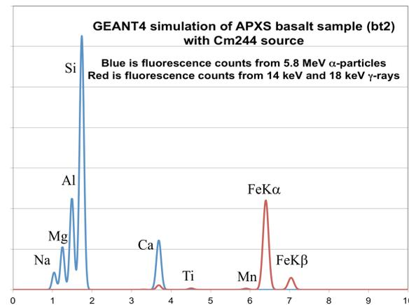
Fig. 3: Simulated spectrum of APXS basalt sample bt2, calculated using GEANT4 and a Fundamental Parameters model of *LunaPIX*. Red spectrum =  $\gamma$ -ray fluorescence, blue spectrum =  $\alpha$ -particle fluorescence (30 mCi <sup>244</sup>Cm).
