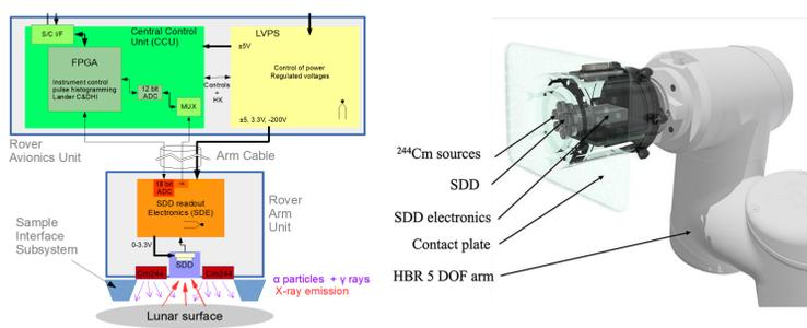
Fig. 1: *LunaPIX* Arm Unit attached to the HoneyBee Robotics robotic arm. During an analysis, a contact plate (translucent in this image) is pressed onto the regolith. An SDD and six <sup>244</sup>Cm sources can be seen recessed from the contact plate.
