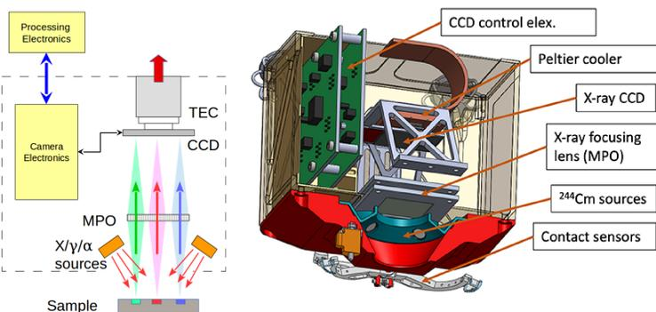
Fig. 2: (left) Fluoresced photons from the sample that are emitted in the direction of a CCD imager are focused by an X-ray lens called an X-ray Micro Pore Optic (MPO) onto the CCD, resulting in a 1:1 image of the sample in its elements. (right) cross-section of the *MapX* flight instrument.
