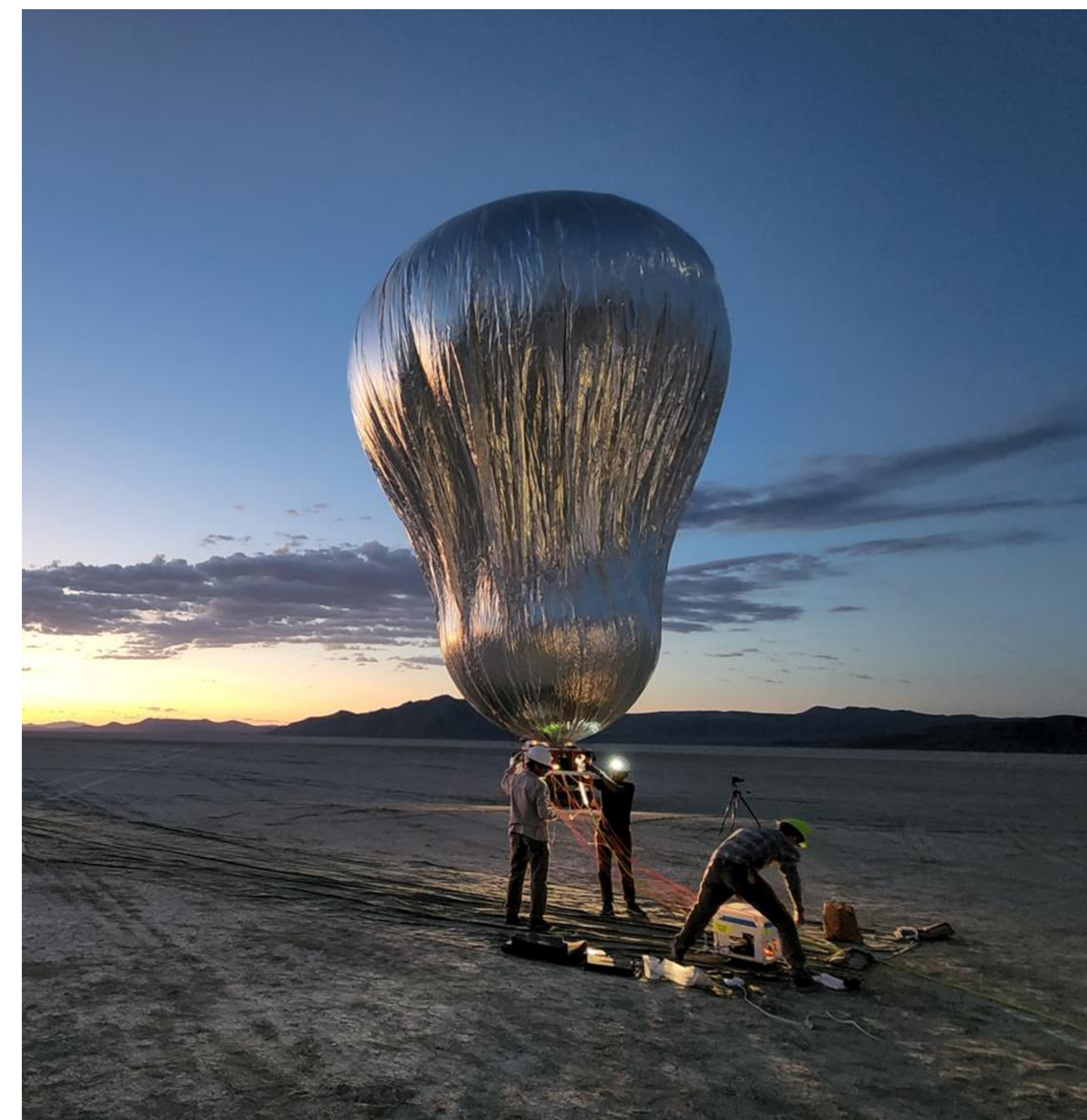
Variable altitude aerobot using buoyancy modulation and Venus compatible envelope material was tested in Nevada's Black Rock Desert in summer 2022. Plans are underway for testing a full scale vehicle.
