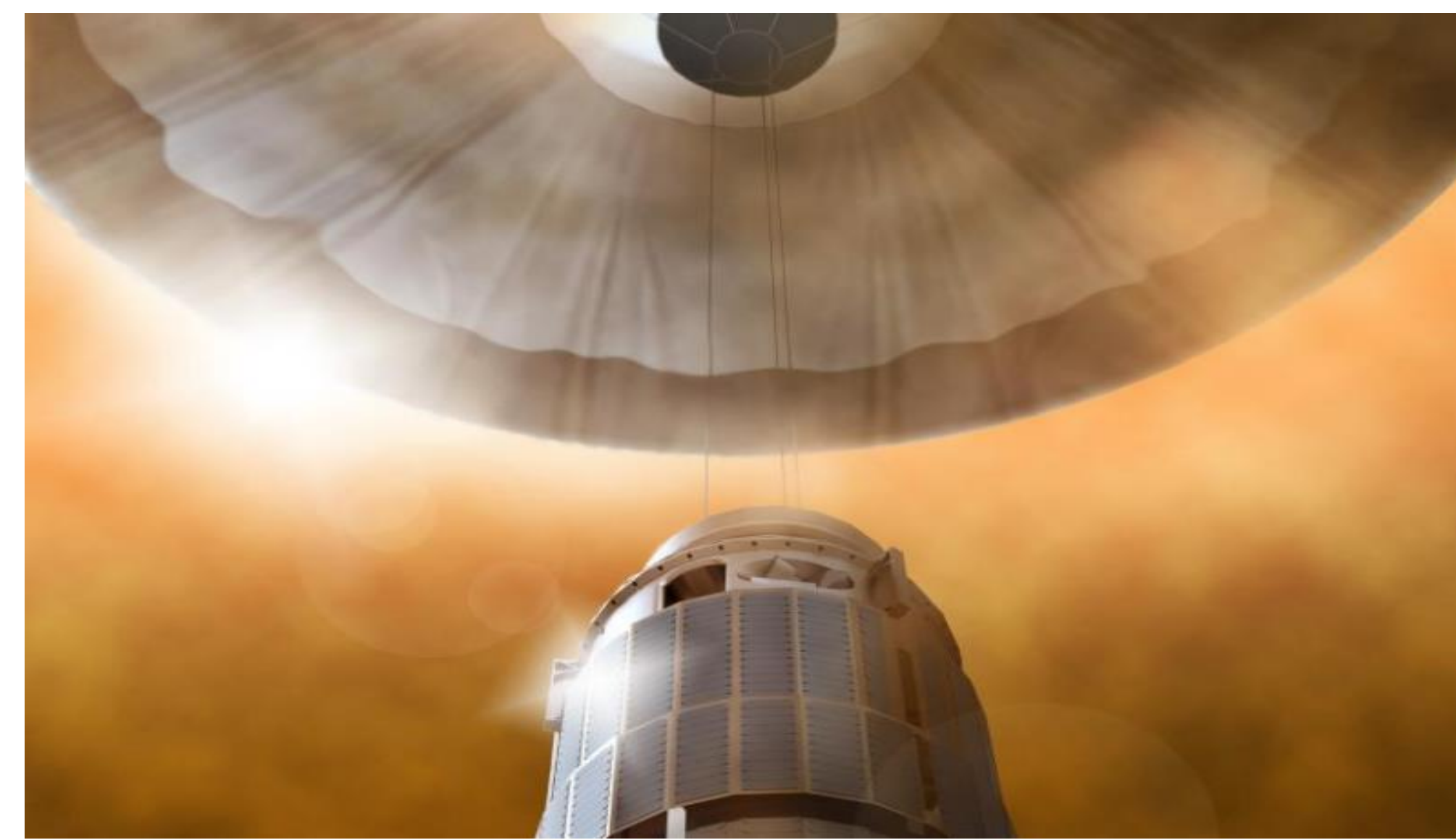
Venus In Situ Cloud Explorer consists of a variable altitude balloon suspending a gondola packed with scientific instrumentation.
