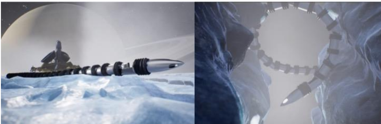
Figure 1 EELS robot for a conceptual Enceladus vent exploration mission as a subpayload of Enceladus Orbilander. The full concept movie is viewable at: https://youtu.be/9E0USzPFE10
