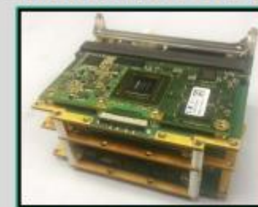
High Speed Processor Module: Power Regulation, FPGA, Data Storage, Multi-core Processor; >250 MB/s write-speed to > 1 TB non-volatile storage; >500 GFLOPs on-board processing
