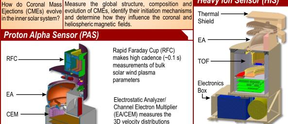
Europe contributes HIS-Electrostatic Analyzer (HIS-EA), which selects alpha particles and heavy ions according to their E/q and elevation angle.
