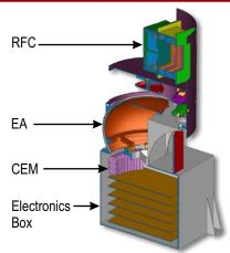
Rapid Faraday Cup (RFC) makes high cadence (~0.1 s) measurements of bulk solar wind plasma parameters
