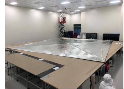
86 m 2 solar sail deployment test
