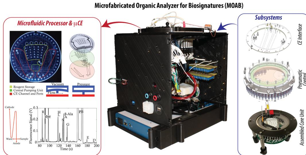
**Figure 1:** Flight-tested MOAB system including a PDMS microfluidic processor, a glass capillary electrophoresis ( $\mu$ CE) wafer, and a laser-induced fluorescence (LIF) detector along with all sensors, electronics and high voltage CE power supplies needed for stand-alone operation.
