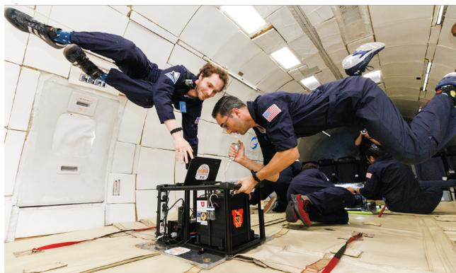
**Figure 2:** In flight view of the MOAB apparatus being operated and monitored under microgravity.
