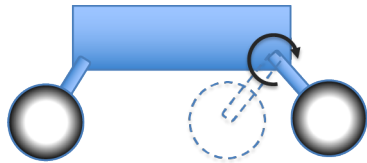
Figure C-2. Four-wheeled skid vehicle with active suspension (amenable to walking).
