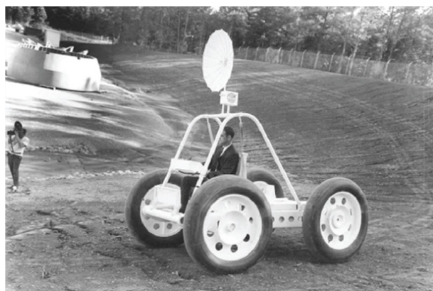
Figure C-5. An example of a lunar rover prototype with different sized front and rear wheels: the Local Scientific Survey Module (LSSM) developed in 1965 by Brown Engineering (NASA).
