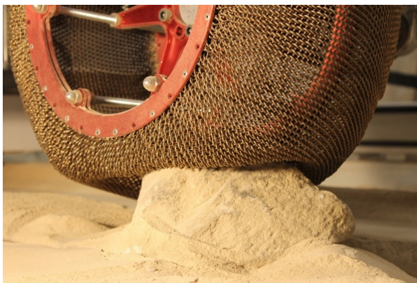
Figure C-2b. Compliant mesh tire referred to as the Spring Tire for its coil-spring interlocking mesh type design inspired by the Apollo LRV wheels.
