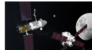
Lunar PPE (Maxar) will use 4 x AEPS engines and 60 kW ROSA arrays
