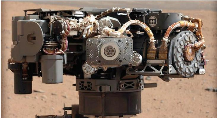
Developed for the Mars Science Laboratory Mission, the Alpha-Particle X-Ray Spectrometer (APXS) is a contact instrument that uses X-ray spectroscopy to determine the elemental composition of soils and rocks. The science objective of the APXS is to produce an understanding of the formation, evolution, and biological potential of the landing site environment through analysis of the variations in elemental composition and distribution of elements comprising the Martian materials.
