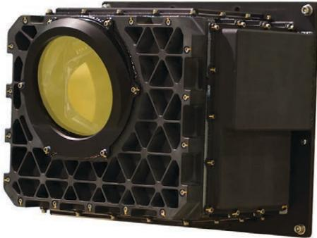
The OSIRIS-Rex Laser Altimeter is a fast scanning lidar system with a single receiver providing 3D point cloud data. OLA was flown in the NASA New Frontiers OSIRIS-Rex Mission and will be responsible for mapping the surface of the Bennu asteroid.
