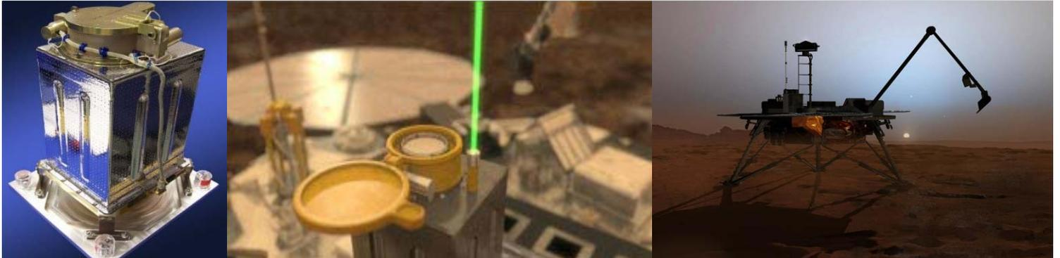
MDA developed the Meteorology package (MET) on the Phoenix Mars Lander, to provide characterization of the Martian climate. The MET consisted of a lidar, three thermocouples and a pressure sensor.
