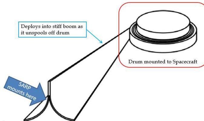
Visualization of the TRAC boom rolling flat on the reel but deploying to generate a more rigid cross section
