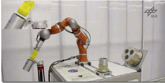
**Exhibit E. Stage 5a – Handling: SARP Inspection and Removal (Ground Command).** A ground-commanded sequence takes a set of inspection images. Once downlinked and reviewed, a ground-commanded sequence has the RA grasp the KINEE interface and remove the SARP from the Inner Sheath. The STS is robust to multiple failures. (Above figure shows the DLR prototype arm removing the SARP during end-to-end testing [§J.10.6.2.2].)
