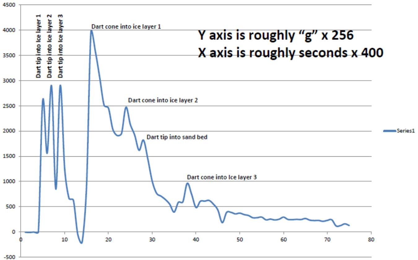
Test results from a Dart dropped from a height of 5m into a layered target at the GSFC Tower Test Facility. The target consisted of a stack of three, 1cm thick, ice sheets separated by 1 inch thick layers of snow resting on a bed of sand. We identified the signals as the Dart tip penetrated each ice layer and then the sand as well as a more degraded signal as the wider conic section of the probe also penetrated these layers.
