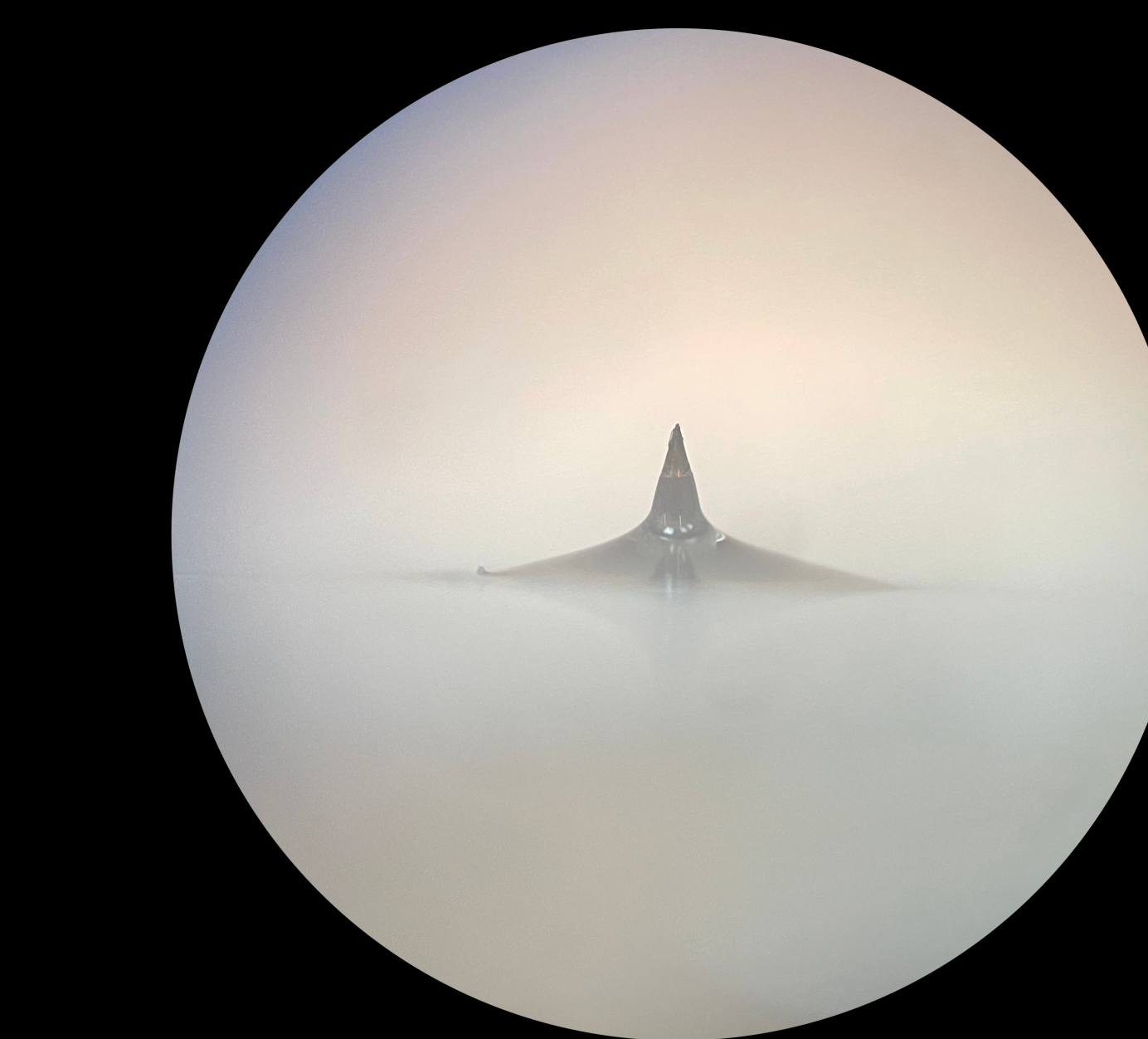
Microscope image of a needle wetted with EMI-BF4
