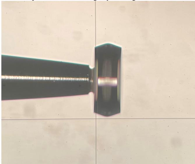
Fig. 2. A test WGM resonator made from lithium tantalate is temporarily mounted on a needle tip for inspection and cleaning.
