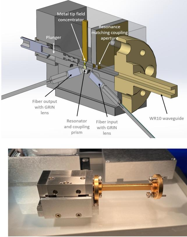
Fig. 1. Conceptual design of the W-band microwave photonic receiver (top) and physical realization of the entire receiver package attached to a standard 94GHz WR-10v waveguide
