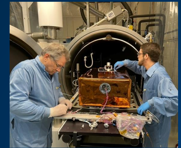
Preparation for Thermal-Vacuum Testing 03/08/2022
