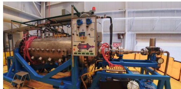
Figure 3. The NTREES at NASA MSFC facility enables low-cost, non-nuclear testing of NTP fuel elements in a flight-like thermal/chemical environment.
